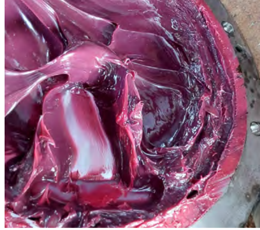
Normally-worn bearing. Purple. G3 wear
