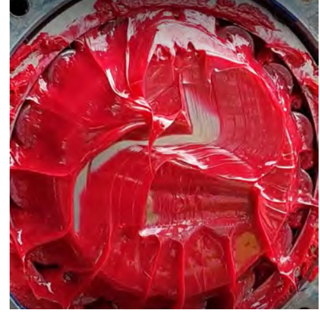
Brand new grease. Bright red. G1 wear
