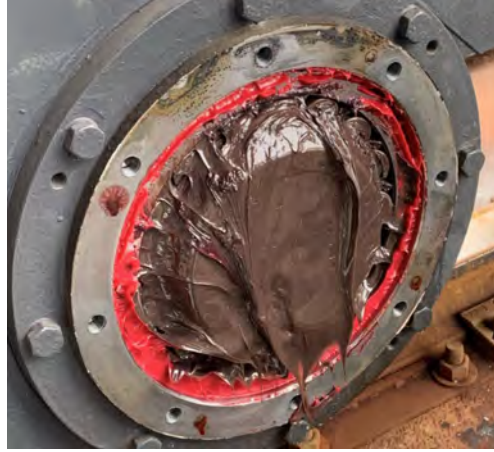
Worn bearing. Purple/brown grease. G4 wear
